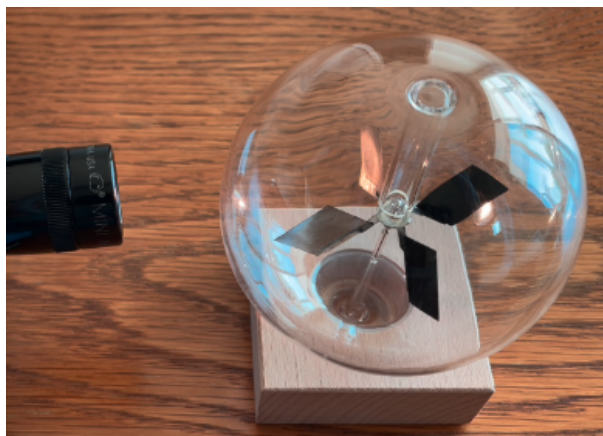
Figure 3: Experiments with light focused on a Crookes radiometer vane.
