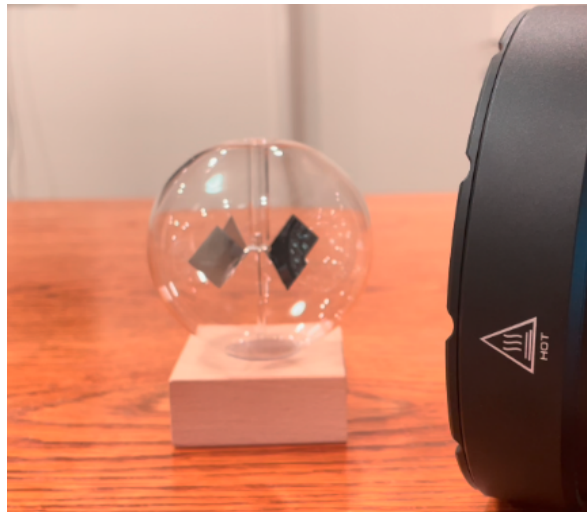
Figure 8: Radiometer rapid heating experiments using a 120,000-lumen flashlight. The videos of the experiments are available on YouTube: The Process Driving Crookes Radiometers and The Force Driving Crookes Radiometers .
