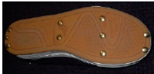
Figure 1. Positioning of the tacks on the sole of the prepared sneakers.
