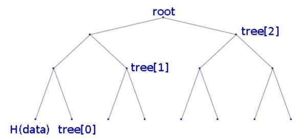
The tree was generated by taking the SHA-256 hash of each user's encrypted data, then concatenating each pair of hashes and hashing that, and repeating this process until reaching the root of the tree.
