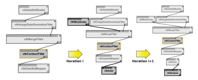
Fig. 4: Predictions are iteratively refined. At each step, a prediction can be extended upstream and downstream; in the second step, the algorithm only suggests a downstream addition. Also, predictions in either direction may include branches in the pipeline, as shown in the center.
