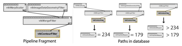
Fig. 5: At each iteration, we examine all upstream paths to suggest a new downstream vertex. We select the vertex that has the largest frequency given all upstream paths. In this example, "vtkDataSetMapper" would be the selected addition.
