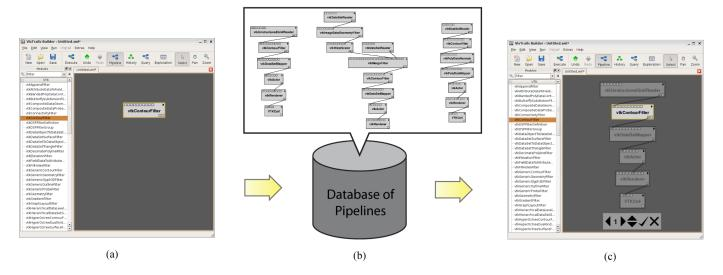
Fig. 1: The VisComplete suggestion system and interface. (a) A user starts by adding a module to the pipeline. (b) The most likely completions are generated using indexed paths computed from a database of pipelines. (c) A suggested completion is presented to the user as semi-transparent modules and connections. The user can browse through suggestions using the interface and choose to accept or reject the completion.
